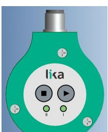
**WARNING** If the START position (START ►) is the same as the END position (STOP ■), the unit resets to factory default settings.
